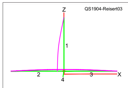
Figure 3 — Current distribution of a quarter-wavelength vertical monopole. Note that for the ground-mounted version, the maximum current and location of the maximum radiation are near the base, where nearby objects can diminish radiation.
